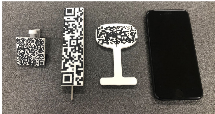
Fig. 2 Markers and smartphone used in the AR-KNEE system. From left to right: guide marker, pointer, oval marker, and smartphone. The camera of the smartphone recognizes two-dimensional bar codes of guide marker, pointer and oval marker when using the AR-KNEE system. Note that the oval marker has a slit that allows the surgeon to mark the tibial rotational alignment reference line
