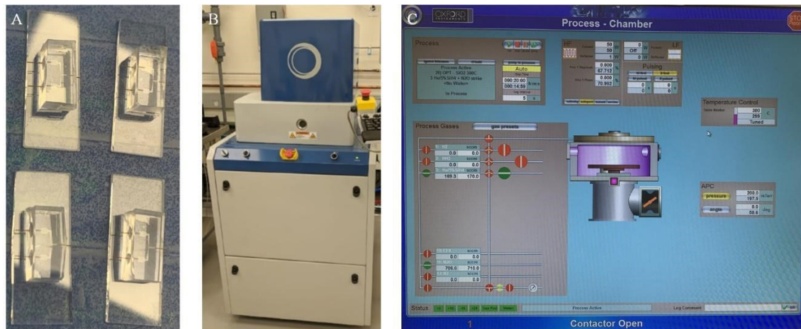
Figure 6. SiO 2 coating. A. Examples of four micromixers fabricated following the above-mentioned step A4. B. PECVD machine of model PlasmaPro ® NGP80. C. Monitoring of the coating process.
