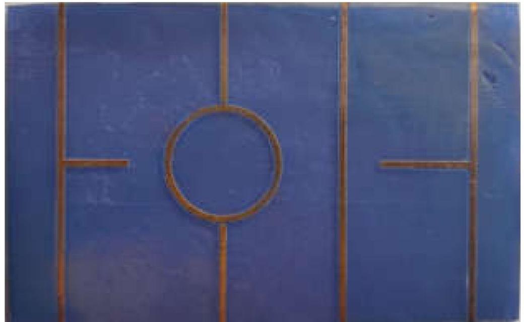
Figure 5. Photograph ( 50 \times 80 mm 2 ) of the calibrating elements employed to measure and extract the electrical parameters of the resin substrate material and the fabrication process. Transmission lines are 850 \mu m wide and 50 mm long, and gaps in the ring resonator network are 360 \mu m.
