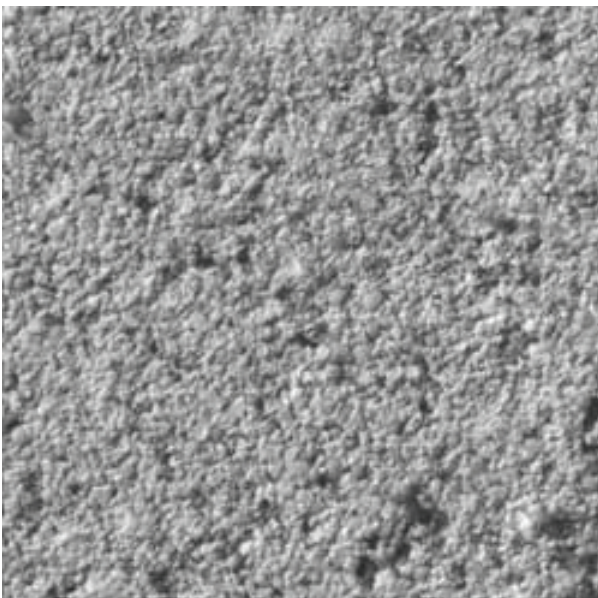
Fig. 1. Scanning electron microscopic image of amalgam surface (without surface treatment) in the control group (magnification, \times 500 ).
