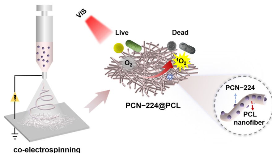
Scheme 1. Schematic diagram of the preparation of the PCL nanofibrous membranes containing PCN-224 NPs (PM NFMs) photodynamic antibacterial NFMs.
