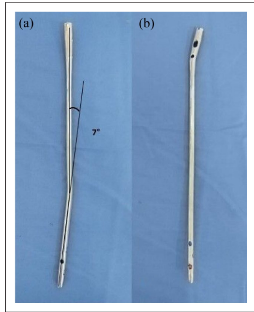
Figure 5. On examination of the removed nail, it was found that the deformity was brought down from 25^\circ initially to 7^\circ in the frontal plane (a), and there was no angulation in the sagittal plane (b).
