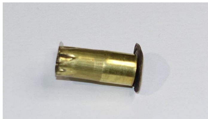
Figure 5. Example of cartridge (AS head stamped) post shot that split at the primer flange.
