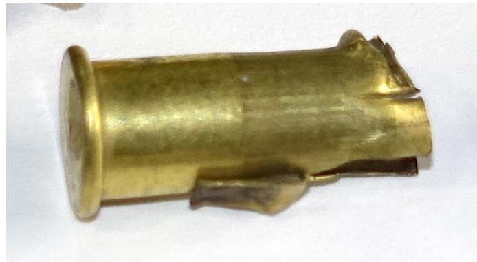
Figure 8. Example of cartridge (AS-head-stamped) post shot that split longitudinally. Note that as in all those that split, the damage terminated at the thicker portion of the case (O.D. Outer Figure 1).
