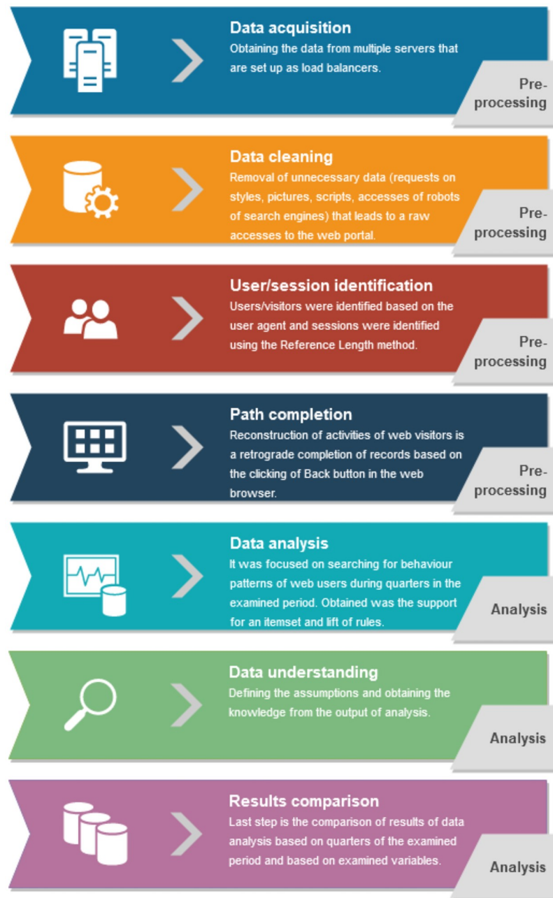
Fig 1. The approach used to process the log files.
