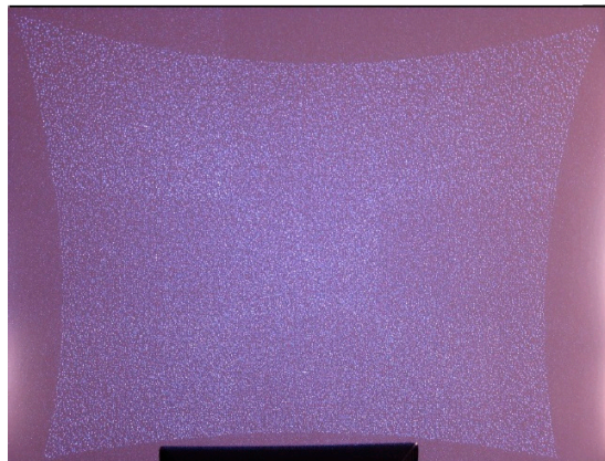
Figure 10. Projected pattern in Light coding.
