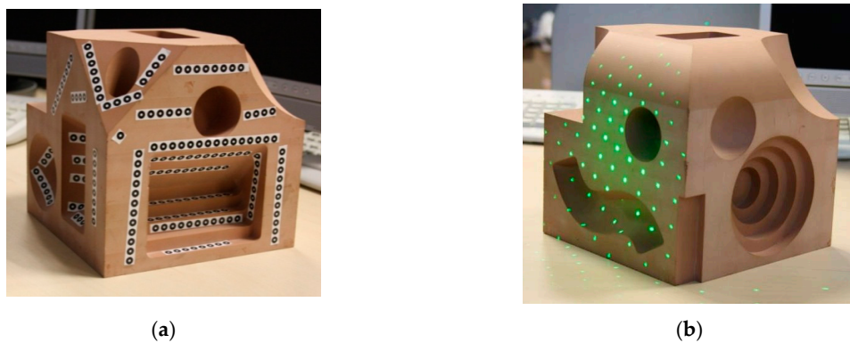
Figure 4. Physical marks used in marker-based stereo vision. (a) Stickers; (b) Laser points.
