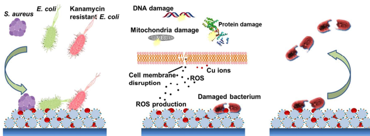
Figure 10 Schematic illustration of the contact killing of bacteria on a Cu-NP incorporated MI-dPG surface coating via the "attract-kill-release" route. Reprinted with permission from Li M, Gao L, Schlaich C, et al. Construction of functional coatings with durable and broad-spectrum antibacterial potential based on mussel-inspired dendritic polyglycerol and in situ-formed copper nanoparticles. ACS Appl Mater Interfaces . 2017;9(40):35411–35418. Copyright (2017) American Chemical Society. 118
