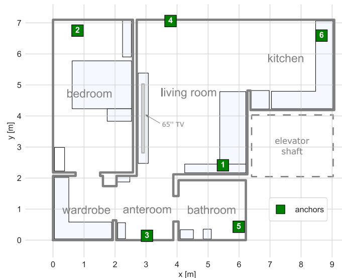
Figure 7. The plan of the experiment area and locations of the system anchors. The blue rectangles mark locations of the furniture pieces and appliances.
