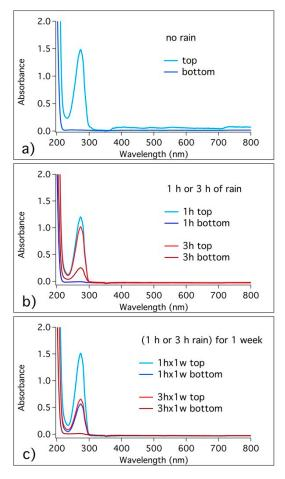
**Figure 9.** UV-vis spectra of the top and bottom piece solutions for surface coated surfaces under different conditions of rain: (a) no rain; (b) 1 h and 3 h of moderate rain; (c) 1 h and 3 h of moderate rain repeated for 1 week.
