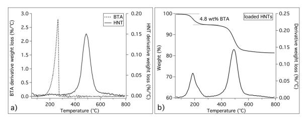
**Figure 2.** Thermogravimetric curves: (a) derivative thermogravimetry (DTG) curves of pristine benzotriazole (BTA) and halloysite nanotubes (HNTs); (b) thermogravimetry (TG)/DTG curves of loaded HNTs, together with the evaluation of BTA weight amount in loaded nanotubes.
