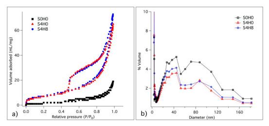
**Figure 6.** (a) Adsorption/desorption isotherms and (b) pore size distribution of S0H0, S4H0, S4H8 and S8H8. Samples have been lyophilized and analysed after 28 days of hydration.
