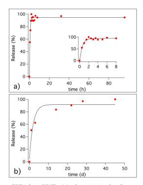
**Figure 8.** Release kinetic of BTA from HNTs: (a) release in simulated pore solution and zoom of the data collected in the first hours; (b) release in S4H8 cementitious formulation. Experimental data are reported as red markers, while black lines represent the exponential curves used to fit the collected data.
