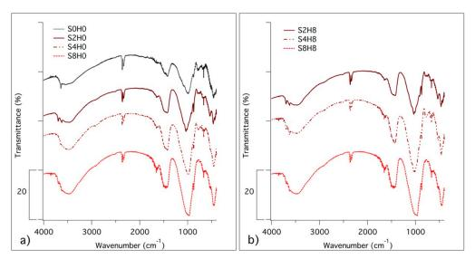
**Figure 4.** FTIR spectra of (a) S0H0, S2H0, S4H0 and S8H0; (b) S2H8, S4H8, S8H8. Samples have been lyophilized and analysed after 28 days of hydration. Spectra have been offset for the sake of clarity.
