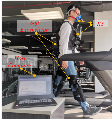
Figure 10. While a subject is walking with the soft exoskeleton, an actuator-driven Bowden cable is used to generate assistance in the lower limb. The metabolic rate is measured through K5.
