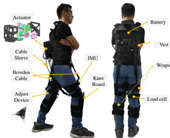
Figure 1. The system overview showing the structure of the soft exoskeleton and the position of each of its parts.
