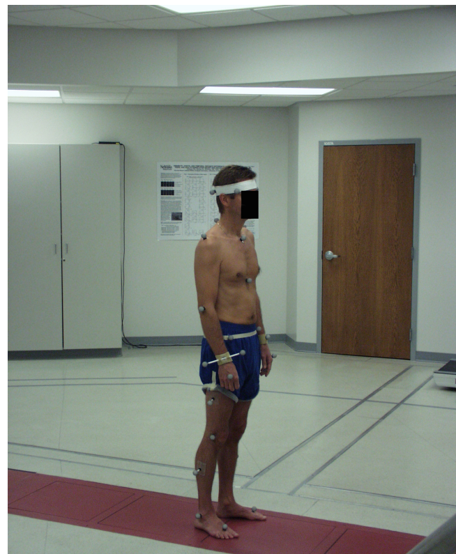
Figure 1 Marker placement for computerized 3-D motion analysis.
