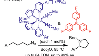
Fig. 1 (a) Examples of bioactive compounds containing \alpha -aryl pyrrolidines. (b) Asymmetric ring-closing C(sp 3 )-H aminations of aliphatic azides to provide non-racemic pyrrolidines.
