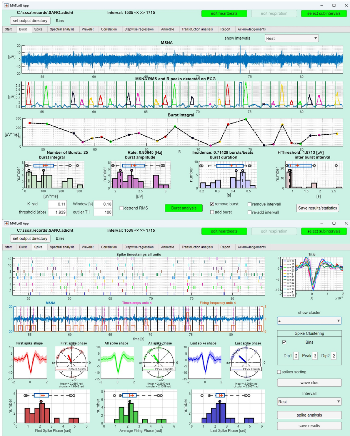
FIG. 4. Burst and spike analysis: (Top) Figure from burst analysis displaying the raw signal, processed RMS signal, and distributions of burst-based metrics; the raw signal is displayed in the first subplot, the processed RMS signal overlaid with green lines indicating the locations of the ECG R-waves in the second subplot, and a temporal series of each burst area calculated in the third subplot. At the bottom the distributions of the burst integral, burst amplitude, burst duration and inter-burst intervals. (Bottom) An output figure from spikes analysis including the raw signal, identified spike events, spikes sorted shapes, and first spike phases for each unit relative to the cardiac cycle.
