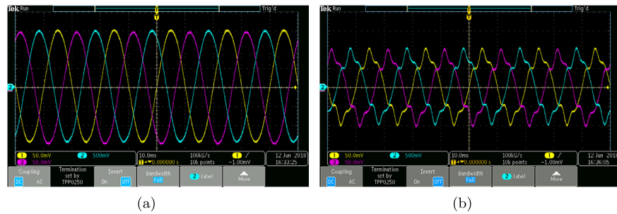
Figure 24. Oscilloscope observation of PSC based compensator (a) Load voltage, (b) Injected voltage.
