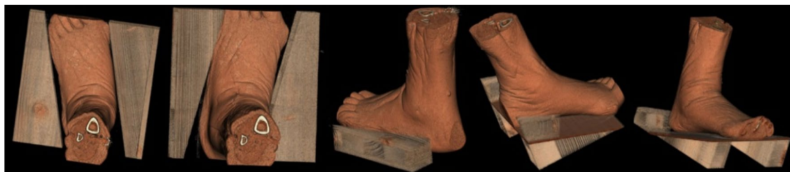
Figure 2. Wooden shanks used to maneuver the specimens in five foot positions in the loading frame during CT scanning; left to right: 15° external rotation, 15° internal rotation, neutral position, 20° plantar flexion, 20° dorsal flexion. The exemplified images are processed via volume rendering using Mimics Innovation Suite (Materialise, Leuven, Belgium).
