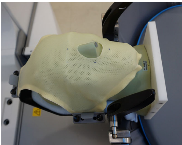
FIG. 3. An anthropomorphic phantom is fixed to the GK Icon with a mask system for a whole procedure test of the accuracy of frameless GKRS.
