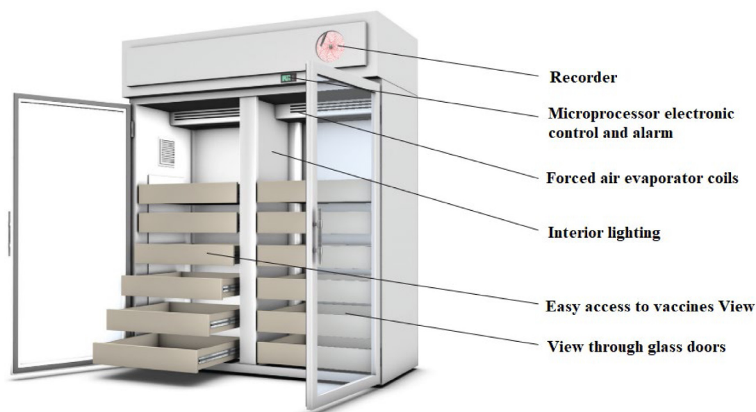
Fig. 5. Refrigerator design used for vaccine storage recommended by the Public Health Unit of Canada (2021).
