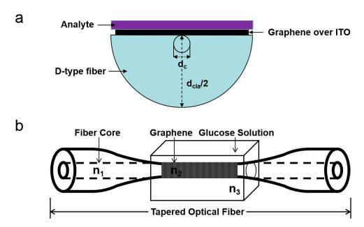
**Figure 4.** (a) Cross-sectional view of the proposed structure. (b) The structure of the tapered optical fiber. Graphene is coated on the core of the fiber.
