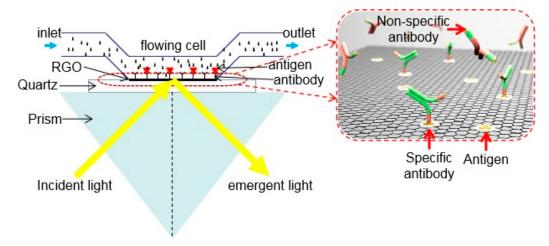
Figure 8. The schematic of reduced graphene oxide (RGO)-based optical sensor.
