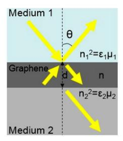
**Figure 5.** Schematic of a graphene layer sandwiched between two dielectrics.
