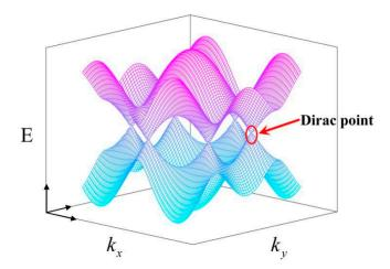
**Figure 1.** Electron band structure and Dirac point of graphene. Purple represents the n-type doped Fermi surface, and light blue represents the p-type doped Fermi surface.
