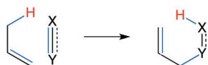
Scheme 2. Alder-ene reaction (XY is, e.g., C 2 H 4 , C 2 H 2 , CH 2 NH, CH 2 O).
