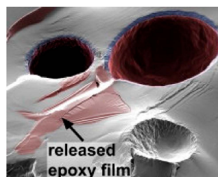
Figure 2. Image of ruptured urea-formaldehyde (UF) microcapsules having both reactive epoxy resin and solvent as the core material. The regions of deposited epoxy film are indicated. Adapted from [12], with permission from © 2009 Elsevier.
