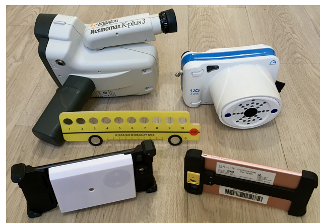
Figure 1 Three vision screening devices. GoCheck Kids (GCK) with flash concentrating case (foreground right) and a second GCK modified with white box containing the nondetailed slowly changing glow fixation device (foreground left). In the background left is the Righton Retinomax, on the right Adaptica 2WIN and center the school bus accommodation-relaxing skiascopy.
