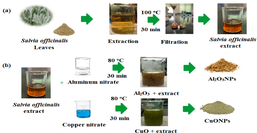
Scheme 1. Biogenic synthesis of metal oxide nanoparticles (a) extraction steps of Salvia officinalis leaves and (b) Synthesis of Al 2 O 3 NPs and CuONPs using Salvia officinalis leaves extract.
