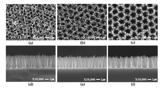
**Figure 3.** FE-SEM images of ZnO nanorod growth on quartz substrate using a PS monolayer template with oxygen plasma treatment. Diameters of polystyrene are (**a**) 800 nm; (**b**) 1300 nm; (**c**) 1600 nm and cross-section of (**d**) 800 nm; (**e**) 1300 nm and (**f**) 1600 nm, respectively.
