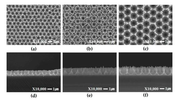
**Figure 4.** FE-SEM images of ZnO nanorod growth on quartz substrate by PS monolayer template without oxygen plasma treatment. Diameters of polystyrene are (**a**) 800 nm; (**b**) 1300 nm; (**c**) 1600 nm and cross-section of (**d**) 800 nm; (**e**) 1300 nm and (**f**) 1600 nm, resepectively.
