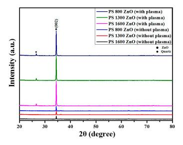
**Figure 2.** X-ray diffraction pattern of ZnO nanorod–assisted PS sphere monolayer arrays grown on a quartz substrate (with and without oxygen plasma treatment).
