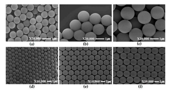
**Figure 1.** FE-SEM images of synthesized PS spheres with diameters of about (**a**) 800 nm; (**b**) 1300 nm; (**c**) 1600 nm and monolayers of (**d**) 800 nm; (**e**) 1300 nm and (**f**) 1600 nm.
