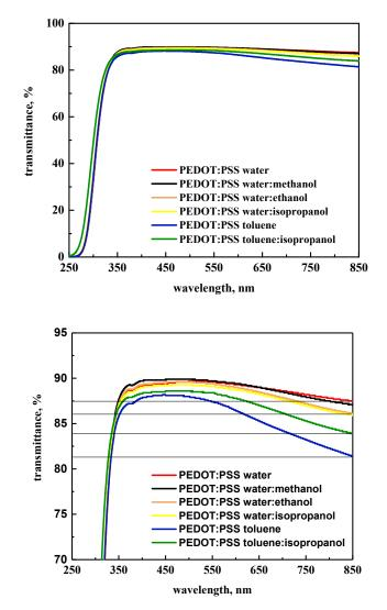
**Figure 7.** UV–Vis spectra of PEDOT:PSS layers in full (top) and from 70% to 95% (bottom) transition mode.
