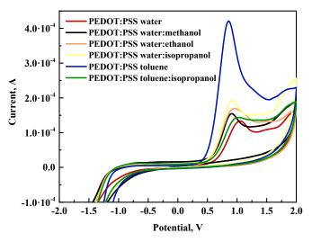
Figure 6. Comparative summary of CV curves for all tested PEDOT:PSS layers.
