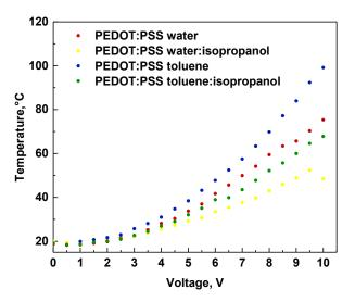
**Figure 9.** The correlation of temperature versus applied potential for constructed devices containing PEDOT:PSS from water, water:isopropanol, toluene, and toluene:isopropanol.
