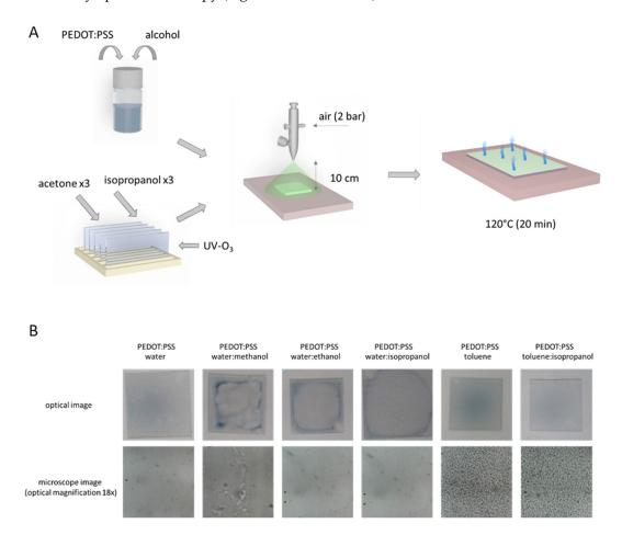
**Figure 4.** Scheme of layer preparation using spray coating technique (**A**); images of PEDOT:PSS layers (spray coated, 10 cm distance, pressure 2 bar) and microscopic images acquired at optical magnification of  $18 \times$  (**B**).
