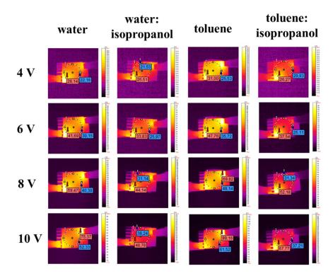
Figure 8. IR images obtained for device architectures (from left to right): ITO/PEDOT:PSS(water)/Ag/ITO,ITO/PEDOT:PSS(water:isopropanol)/Ag/ITO,ITO/PEDOT:PSS(toluene)/Ag/ITO,andITO/PEDOT:PSS(toluene:isopropanol)/Ag/ITO at 4.0 V, 6.0 V, 8.0 V, and 10.0 V.
