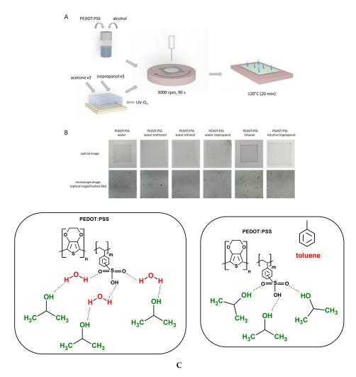
**Figure 2.** Scheme of layer preparation using spin coating technique (**A**); images of PEDOT:PSS layers (spin coated at 3000 rpm, 90 s) and microscopic images acquired at optical magnification of  $18 \times$  (**B**); scheme of primary and secondary hydrogen bond interactions of PEDOT:PSS in water and toluene with isopropanol (**C**).
