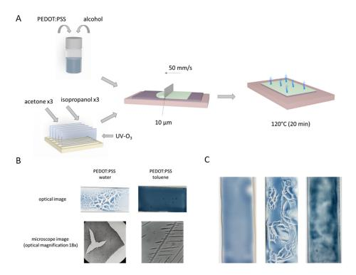
**Figure 3.** Scheme of layer preparation using doctor blade technique (**A**); images of PEDOT:PSS layers (10  $\mu$ m gap, 50 mm/s) and microscopic images acquired at optical magnification of 18× (**B**); PEDOT:PSS (from water) layer (from left to right): directly after casting, after annealing, and layer made from PEDOT:PSS (from water:isopropanol) layer after annealing (**C**).
