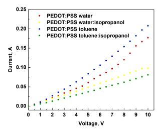
**Figure 10.** The correlation of current with applied potential for constructed devices containing PEDOT:PSS from water, water:isopropanol, toluene, and toluene:isopropanol.
