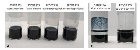
**Figure 1.** Poly(3,4-ethylenedioxythiophene:poly(styrenesulfonate) (PEDOT:PSS) in water or toluene mixed with different alcohols: methanol, ethanol, and isopropanol ((**A**)—stable mixtures, (**B**)—unstable mixtures).
