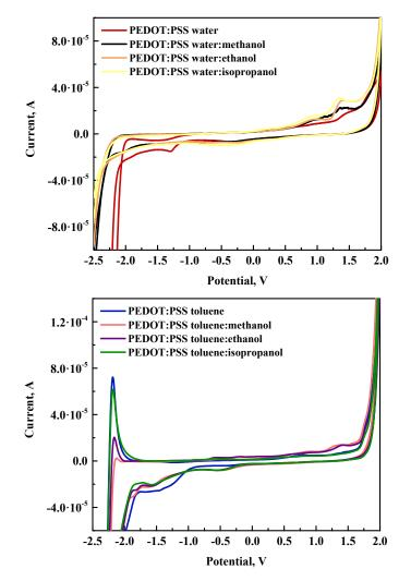
**Figure 5.** Comparative cyclic voltammetry (CV) curves for PEDOT:PSS in water (top) and toluene (bottom).
