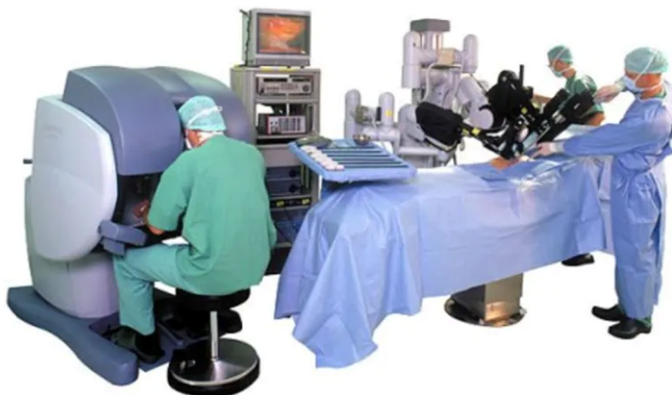
Figure 1. The da Vinci classic teleoperated surgical system, which is still a popular platform for RAMIS research, due to the DVRK extension. Image credit: Intuitive Surgical.
