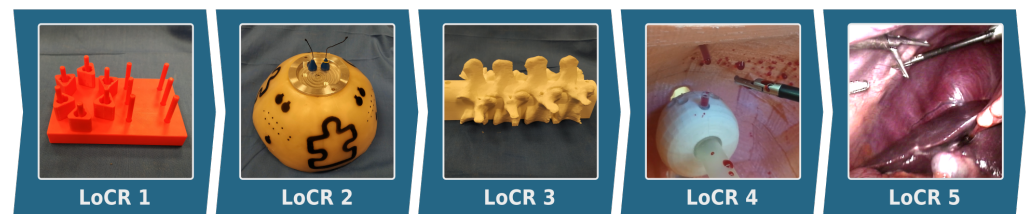
Figure 2. The Level of Clinical Relevance (LoCR) scale for Robot-Assisted Minimally Invasive Surgery (RAMIS) with examples. LoCR 1 : 3D printed board for the peg transfer training task, designed by Hwang et al. [27]; LoCR 2 : Fundamentals of Robotic Surgery (FRS) training dome; LoCR 3 : 3D printed bone phantom for drilling tasks; LoCR 4 : anatomically relevant silicone pelvis phantom [36]; LoCR 5 : in vivo human surgical environment [37].
