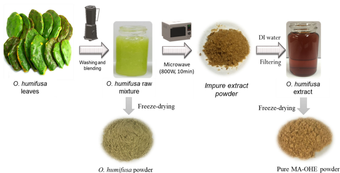
Figure 1. Schematic illustration of the microwave-assisted O. humifusa extract (MA-OHE) process.
