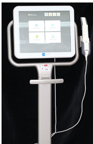
Fig. 1 Intraoral scanner (iTero Element 2; Align Technologies) Abb. 1 Intraoralscanner (iTero Element 2; Align Technologies)
