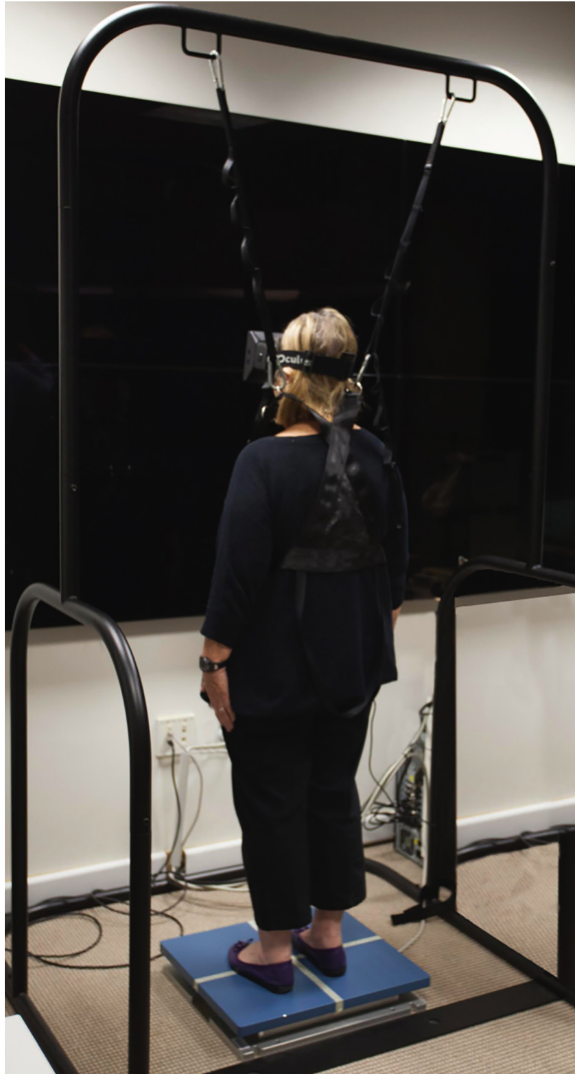
Fig 2. Patient performing the test on the virtual reality environment, while standing on the force platform and wearing the head-mounted goggles.
