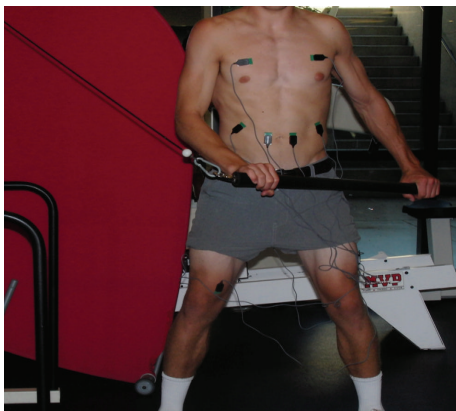
FIGURE 1: Surface EMG setup for wood chop cable pull exercise.
