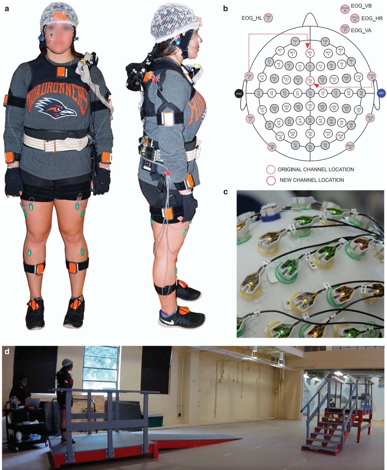
Figure 1. Fully instrumented subject and experimental gait course. (a) Able-bodied subject instrumented with EEG, EMG, and full-body motion capture. (b) EEG channel montage and EOG locations. EOG_HL: horizontal left, EOG_HR: horizontal right, EOG_VA: vertical above, EOG_VB: vertical below. (c) Close-up image of active EEG electrodes. (d) Experimental gait course including level walking, ramps, and stairs.
