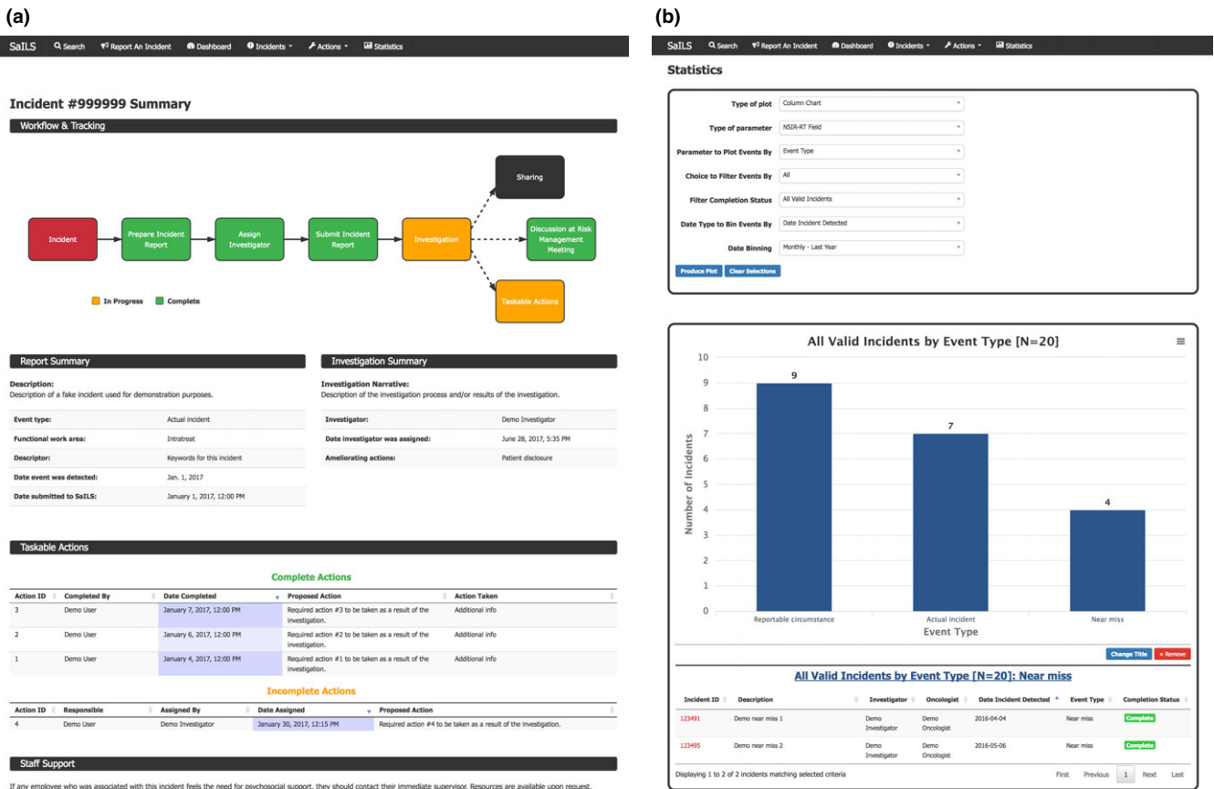
Fig. 5. Screenshots of the incident tracking functionality and data visualization interface of SaILS. (a) Example incident summary: A dynamic flowchart depicting the current status of the incident investigation is included at the top of the page. Relevant report and investigation details are provided in tables below the flowchart. All taskable actions (a user-requested feature) associated with the incident are listed in additional tables underneath. (b) Data visualization interface: A form is provided at the top of the page that allows users to specify plotting parameters. An example column chart of incidents distributed by the Event Type data element is shown. The list of near miss incidents underneath the plot was generated by clicking the near miss column; a feature which was requested by users.
