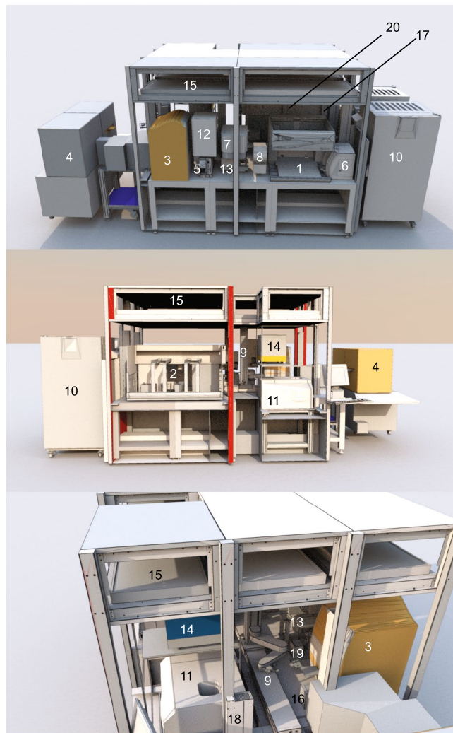
Figure 1. Schematic of the automated platform. (1) Liquid handler Biomek NX Span-8 including the plate shaker Shaking Peltier ALP and a tilting station Amplius (AIG) 3D Tilting ALP, (2) Liquid handler Biomek FXP (96- and 384-pipetting head including active wash-station and a BioShake 3000), (3) Acoustic droplet ejector Labcyte Echo550, (4) High content imager Yokogawa CV8000, (5) plate sealer Wasp, (6) Cell counter Vi-Cell XR12, (7) plate seal remover Nexus Xpeel, (8) Barcode printer and reader Scinomix Sci-Print MP2, (9) Precise SCARA robotic arm on rail, (10) 4 °C and 37 °C incubators Cytomat 24-C, (11) Sigma refrigerated centrifuge 6-16KR, (12) Tube de-capper Cap-it All, (13) Plate washer Biotek 405 LSHTV, (14) Multimode plate reader SpectraMax i3 Multi-Mode Platform and Minimax imager, (15) Custom made biosafety class 2 enclosure, (16) 2D-barcode reader Visionmate, (17) 4 deliidding modules, (18) 5 Tipbox labware feeders, (19) Regrip station, (20) 4 shelf labware hotel.
