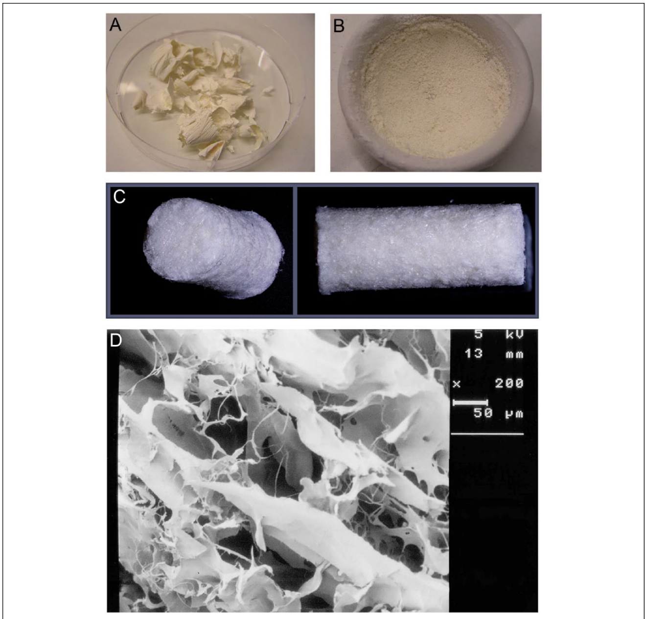
Figure 1. The production of the scaffolds starts with lyophilized cartilage shrapnels ( A ) that were ground into small particles ( B ) that are subjected to several enzymatic treatments. The produced scaffolds are porous ( C ), as was confirmed by scanning electron microscopy ( D ). The scale bar represents 50 \mu\text{m} .
