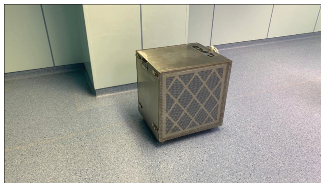
Figure 1: Portable HEPA filter
