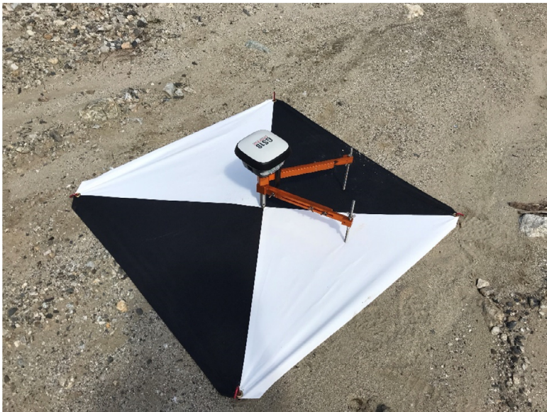
Fig. 3. Photograph of a typical \sim 1 \text{ m}^2 ground control points (GCP) target. The vinyl targets were secured to the ground using tent stakes. The photograph also shows the Leica GS-18 GNSS antenna on an orange colored portable "spike mount" used to measure the precise center location of the GCP.
