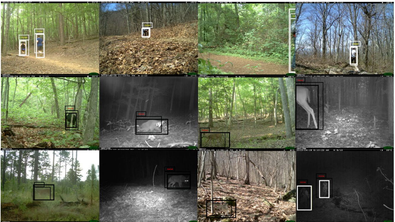
FIGURE 6 Example detection result of our proposed algorithm classifying humans in white bounding box and animals in black. These show that our method can handle challenging conditions including object deformation, occlusion, and low contrast. A misclassification sample is shown in the last row. Thin and bold border bounding boxes refers to our results and ground-truth, respectively
