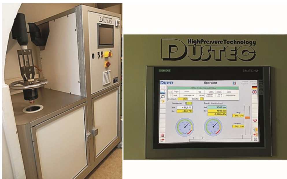
Figure 5. Pressure testing system (HighPressureTechnology Dustec, Wismar, Germany), with a sample volume of 200 mL. High hydrostatic pressures up to 600 MPa can be applied. Temperatures between 0 °C and 40 °C can be set constantly during HHP treatment.
