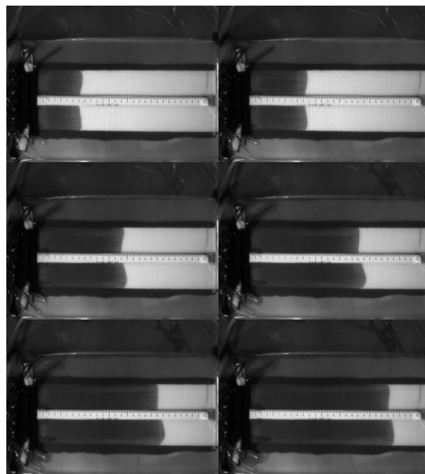
Figure 14. Flow visualization of RTM using a seven-layer fiber preform: images captured at the 50th, 100th, 150th, 200th, 250th, and 300th second.
