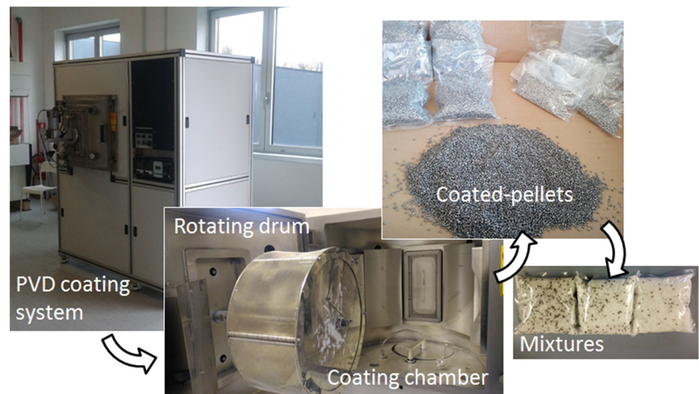
Figure 1. PVD coating systems and coated pellets.
