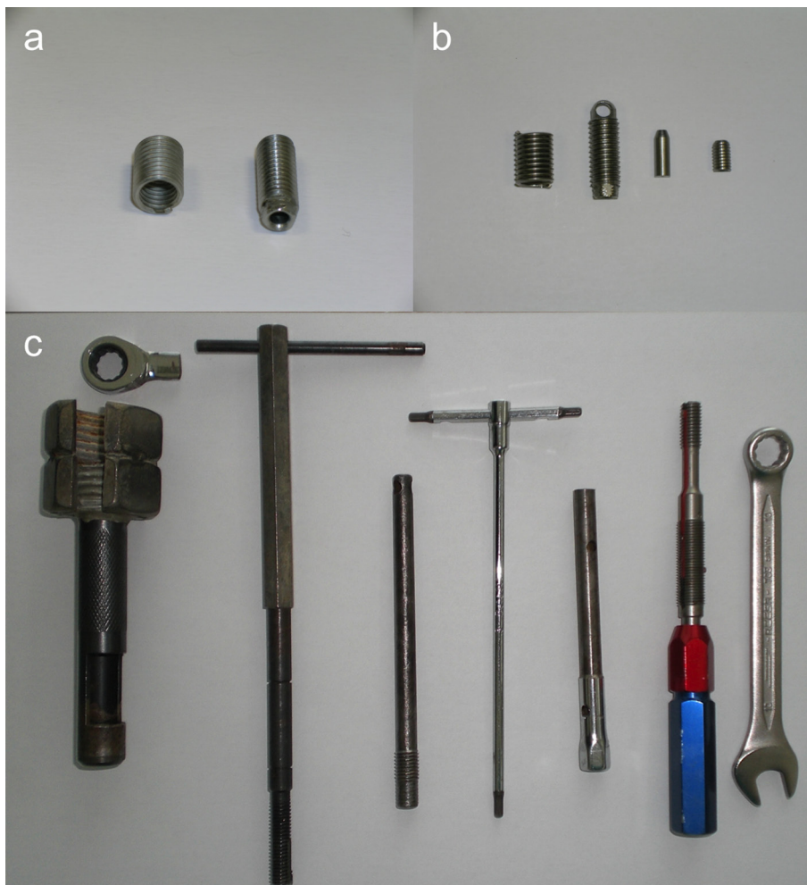
Fig. 1. From left to right: (a) helicoil and tibial screw; (b) helicoil, femoral screw, piston, and push screw; (c) modified pre-winder with ratchet, threaded mandrel, guided tape, hex key, socket wrench, extractor, open end wrench.
