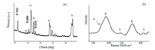
**Figure 3.** Grazing incidence X-ray diffraction (GIXRD) spectrum (**a**) and Raman spectrum (**b**) of titania nanowires (TNW4) obtained during the thermal oxidation of Ti6Al4V with the use of  $Ar/H_2O_2$ , T = 500 °C.
