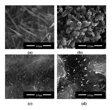
**Figure 2.** SEM images of titania nanoneedles (TNN3, (**a**)), titania facetted crystals (TNN2 (**b**)), and titania nanowires (TNW1 (**c**)) and (TNW6 (**d**)).
