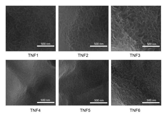
**Figure 1.** Scanning electron microscopy (SEM) images of titania nanofibers (TNF, produced by the direct oxidation of Ti6Al4V substrates, using H<sub>2</sub>O<sub>2</sub> (TNF1, TNF2, TNF3) and H<sub>2</sub>O<sub>2</sub>/CaCl<sub>2</sub> agents (TNF4, TNF5, TNF6).
