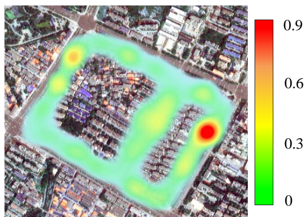
Figure 11. Gas Supply System Risk Heatmap Monitoring. Please note that the business users are usually distributed along the street and here we only draw the gas supply system risk for every business user.
