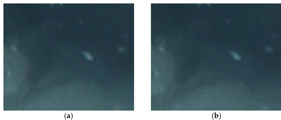
Figure 5. Received underwater image 3 signals using 4-QAM with the CEE of 10% and transmission BERs of 10^{-3} and 10^{-4} , respectively. ((a): PSNR = 34.73 dB; (b) PSNR = 45.64 dB).
