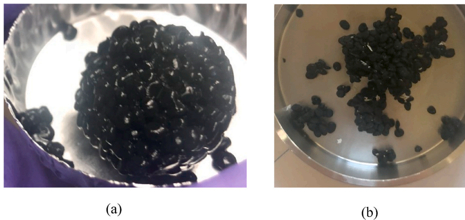
Fig. 1. Granules: (a) saturated, ready to be mixed with soil after homogenization, and (b) at 3% relative humidity (RH).
