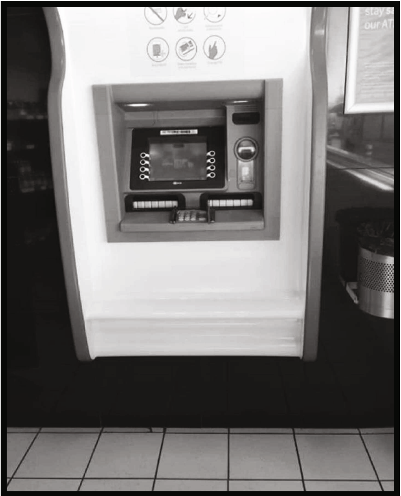
FIGURE 2: Automated teller machine that is not user friendly to persons with visual impairment (figure recoloured to prevent identification of the service provider).
