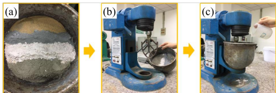
Figure 5. The process of preparing reactive powder concrete: (a) put the dry powder into the container; (b) stir the dry powder; (c) add water for further stirring.
