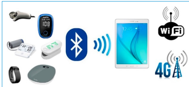
Figure 3. E-care's connected non-intrusive medical sensors.
